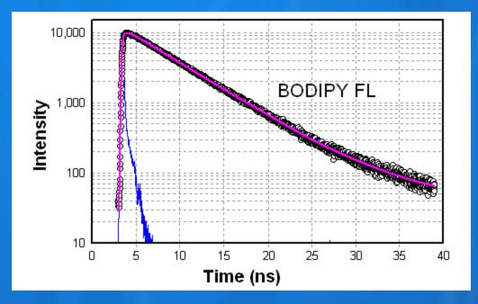
$λ_{Ex}$ : 447-nm Diode Laser Em: KV 505 LP τ = 5.66 ns (water)
